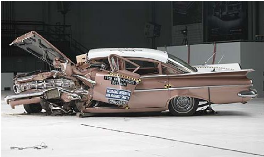
The passenger compartment of the '59 Bel Air is greatly deformed
