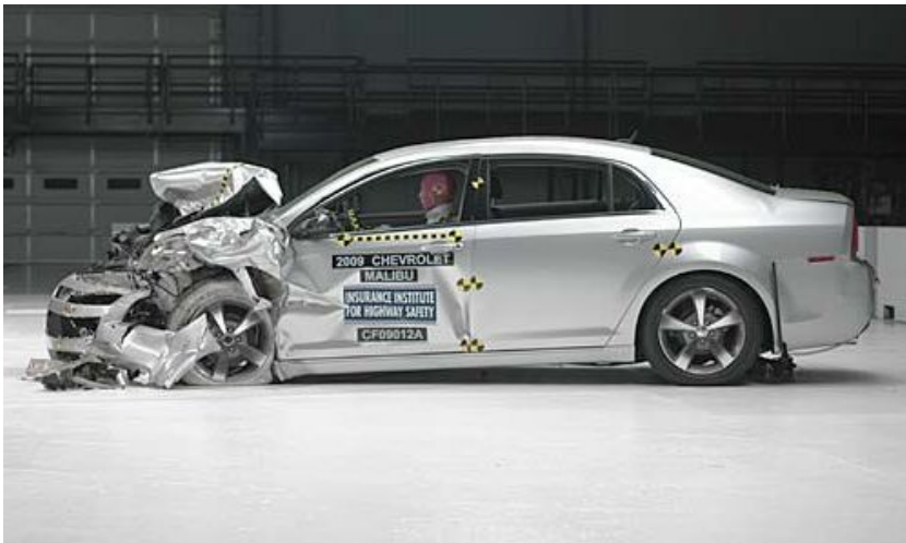
Passenger compartment of the '09 Malibu stays completely intact
