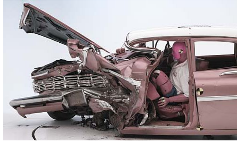
The passenger compartment of the '59 Bel Air is greatly deformed
