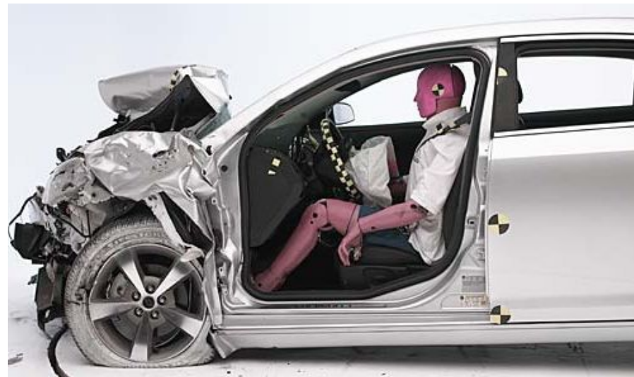
Passenger compartment of the '09 Malibu stays completely intact
